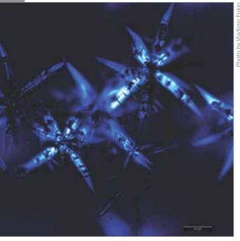
Orchid-like crystals in the interior of CaO-Li<sub>2</sub>O-SiO<sub>2</sub> glass.
