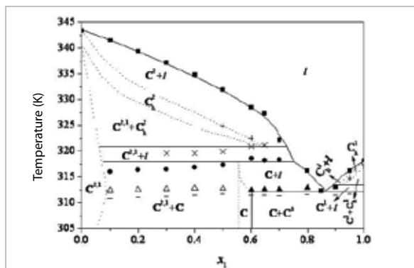
Figure 2. Phase diagram for the system lauric acid (1) + stearic acid (2). (■) fusion temperature; (●) peritectic temperature; (▲) eutectic temperature; (×) metatectic temperature; (+), (Δ), (-) transitions temperatures on the solid phase; (○) transition on the solid phase of the pure component (Costa et al., 2009)
