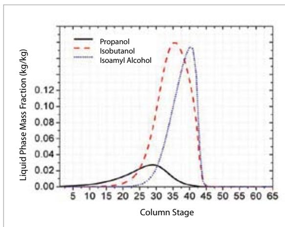
Figure 1. Concentration profiles of high alcohols in bioethanol distillation columns BB1 (Batista and Meirelles, 2009)
