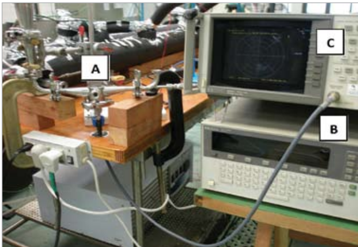
Figure 1. Assembly for continuously testing dielectric properties of the sugarcane must as functions of temperature: (A) probe cell; (B) connecting cable; (C) network analyzer
