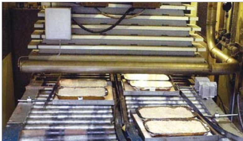
Figure 1. Sugarcane bagasse irradiation in batch system at the Electron Beam Accelerator in the Nuclear and Energy Research Institute, IPEN. (Photo Jesus Carlos/Imagemlatina)
