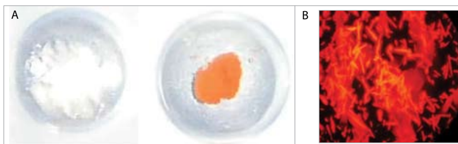
Figure 1. (A) Photographs showing the mesoporous catalyst MCM-41 before (left) and after (right) modification with the photosensitizer PDI. (B) Optical micrograph of the modified mesoporous catalyst, registered with an inverted fluorescence microscope, showing the strong red emission of the incorporated dye
